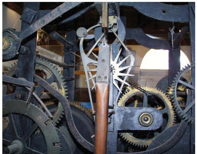
Figure 11: 14-legged gravity escapement of clock 6.
