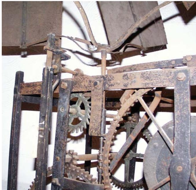
Figure 6: The unusual striking work of clock 4.
