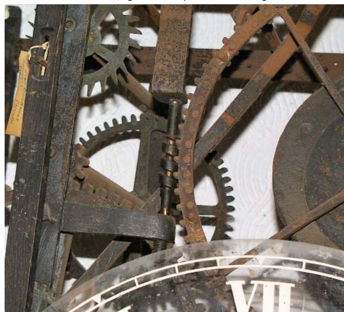
Figure 7: The worm drive to the fly of clock 4.
