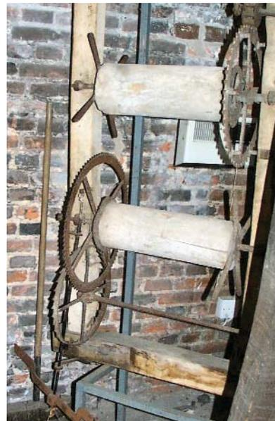
Figure 2: Ramsey movement showing the restored verge.
