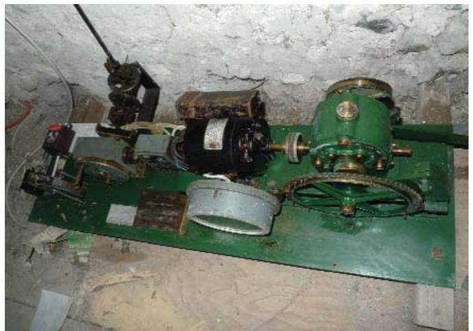
4. Gillett's synchronous clock. From left: strike let-off switch; time gearbox; synchronous motor; strike stop switch and motor; strike gearbox and countwheel.
