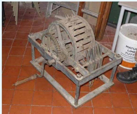
Figure 9. Chiming machine at Wethersfield.
