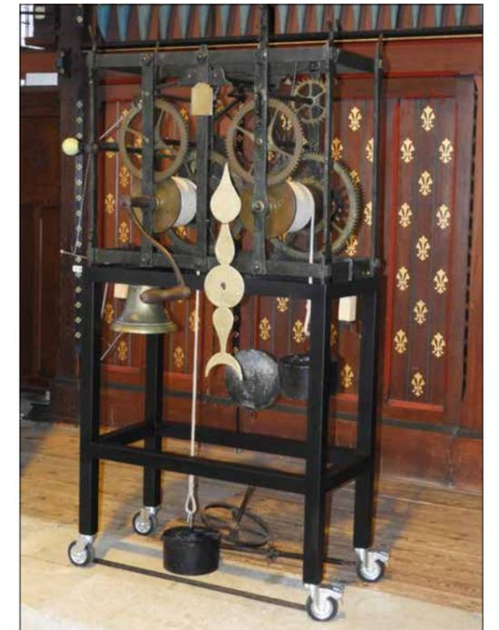
Figure 21. Hutley's countwheel with let-off pins.
