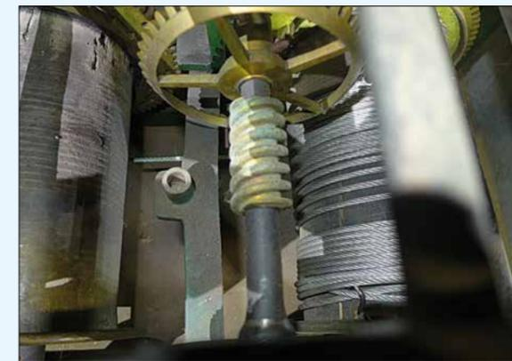
Figure 12. Worm drive on the Terling clock.
